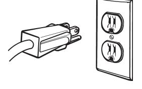
A **TEMPORARY** adapter may be used to connect the charger to a two-pole outlet if a properly grounded outlet is not available. Use the adapter **ONLY** until a properly grounded outlet can be installed by a qualified electrician.
